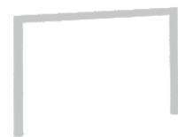
Tubular: CRCA Pipe, 50 diameter, 40 horizontal square pipe
